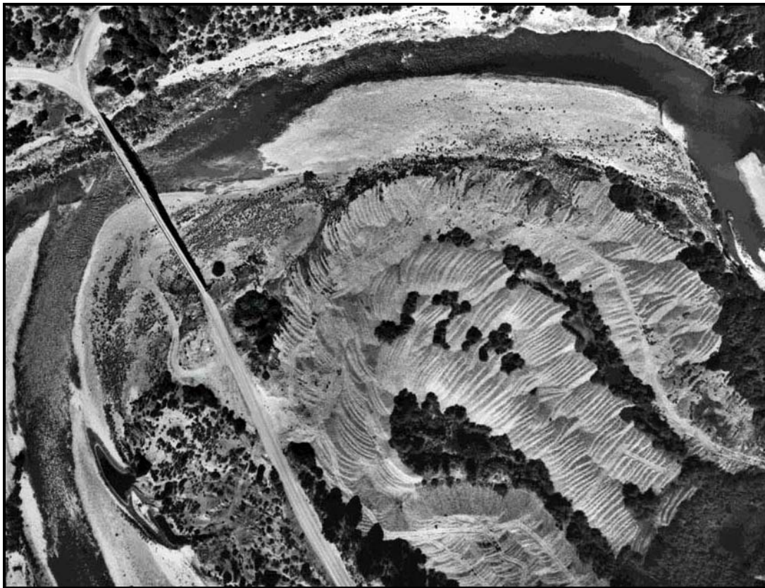
Photo 3-2 Example of rock tailings showing amount of alluvium moved by dredgers. Photo taken near Junction City in 1961
